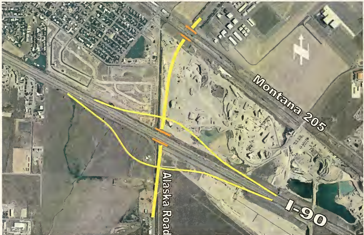
Figure 2-1 Conventional Diamond Interchange
